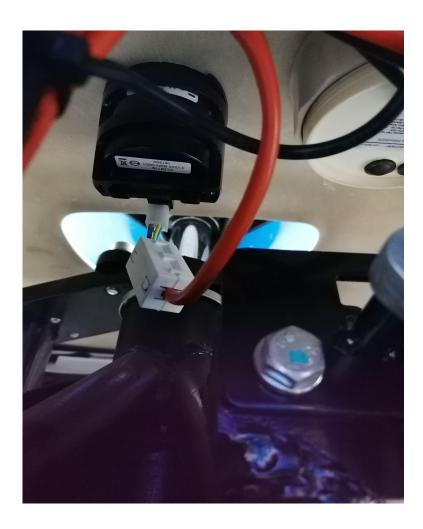
Clamp the ferrite filter (supplied by ETF) on all 4 wires together close to the back of the BDI. Add a little tie-wrap behind the ferrite to keep it in place.
