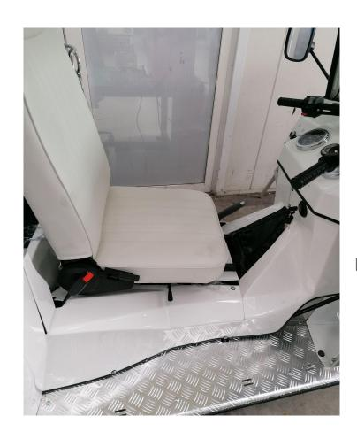
Remove the driver's seat. Remove the black bag and the lower plate from the driver's seat (both fastened with Velcro). Remove the fiber cover panels on the right side (remove screws). For assembly, do the reverse process.
